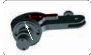
Place the rotation unit with the linear guide back on the tube. Note that the rotation stop fits between the two locking pins at the top. Tighten the bolt until it is attached to the rotation element on the inside. Now turn the bolt three strokes and tighten the lock nut for security reasons.
