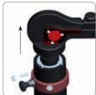
On top of the tube, there is a pattern of holes (a) where small metal pins (b) can be placed.
