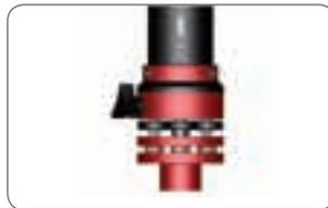
4) Rotate the counterweight using a small screwdriver, until the socket screw of the counterweight is accessible.
